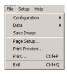
The file menu allows the user to load or save a data record or configuration file as well as print the current display. Data is stored as an ASCII file in commaseparated value (CSV) format. Configuration files are binary.
