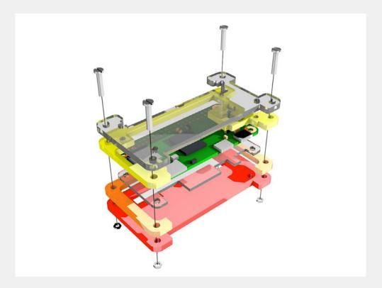
The first thing to do, is to peel off the protective film from all of the Perspex layers.
