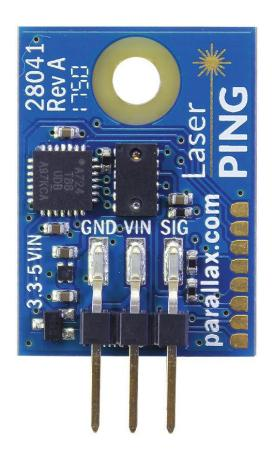
The sensor's built-in co-processor ensures the right logic levels. Its I/O connections operate at the same voltage supplied to the VIN pin, for compatibility with 3.3V and 5V microcontrollers.
