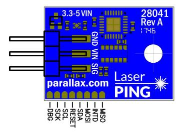
End-user access of the test pads, beyond changing the default mode upon startup from PWM to Serial, is not supported.
