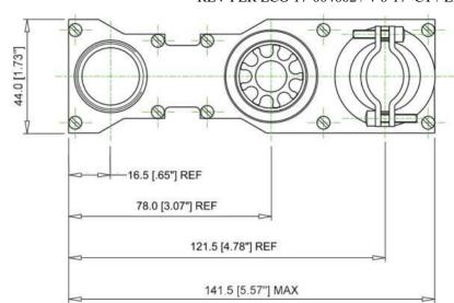
END VIEW WITH ITEM 4 CABLE CLAMP DELETED FOR CLARITY
