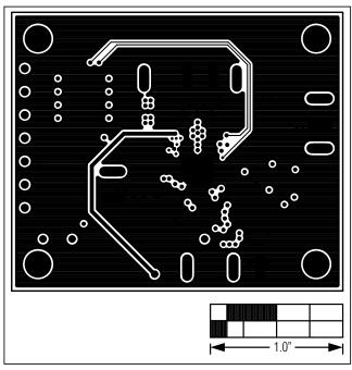
Figure 5. MAX17019N EV Kit PCB Layout—Layer 3
