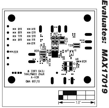
Figure 7. MAX17019N EV Kit Component Placement Guide— Solder Side
