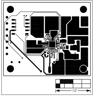
Figure 3. MAX17019N EV Kit PCB Layout—Component Side
