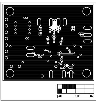
Figure 4. MAX17019N EV Kit PCB Layout—Layer 2
