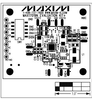
Figure 2. MAX17019N EV Kit Component Placement Guide— Component Side
