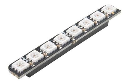
**Description:** The Pimoroni Blinkt! is a "shield" for the Raspberry Pi, equipped with eight superbright and addressable RGB LEDs that make it ideal for adding visual notifications to your Pi. Each LED is individually controllable and dimmable, allowing you to create gradients, pulsing effects, or just flash them on and off like crazy.
