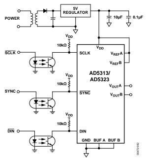
Figure 37. AD5313/AD5323 in an Opto-Isolated Interface
