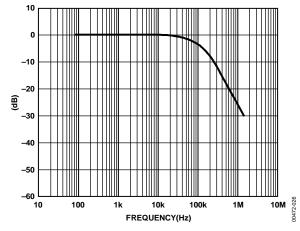
Figure 22. Multiplying Bandwidth (Small Signal Frequency Response)
