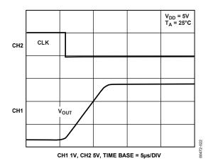
Figure 18. Half-Scale Settling (¼ to ¾ Scale Code Change)
