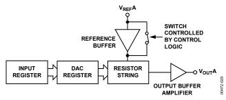
Figure 25. Single DAC Channel Architecture
