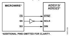
Figure 33. AD5313/AD5323 to MICROWIRE Interface
