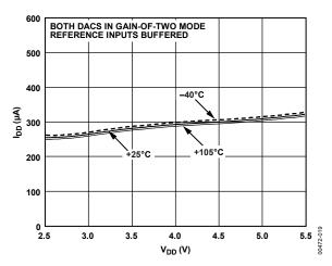
Figure 15. Supply Current vs. Supply Voltage
