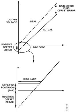
Figure 2. Transfer Function with Negative Offset
