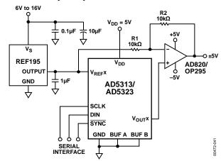
Figure 36. Bipolar Operation Using the AD5313/AD5323
