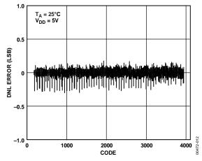
Figure 10. AD5323 Typical DNL Plot
