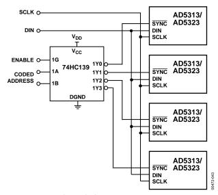
Figure 38. Decoding Multiple AD5313/AD5323 Devices in a System
