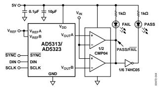
Figure 39. Window Detector Using AD5313/AD5323
