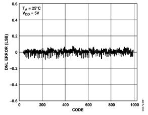
Figure 9. AD5313 Typical DNL Plot
