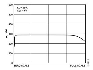
Figure 14. Supply Current vs. Code
