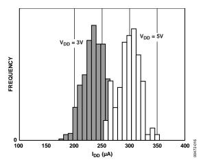
Figure 12.  $I_{DD}$  Histogram with  $V_{DD} = 3 V$  and  $V_{DD} = 5 V$
