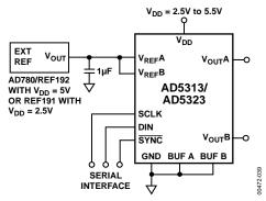
Figure 34. AD5313/AD5323 Using External Reference
