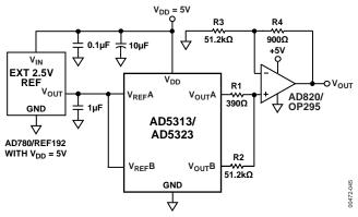
Figure 40. Coarse and Fine Adjustment
