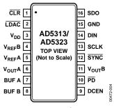
Figure 6. Pin Configuration
