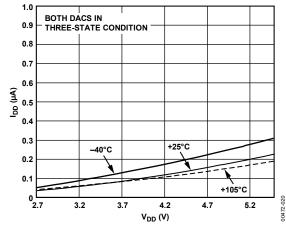
Figure 16. Power-Down Current vs. Supply Voltage
