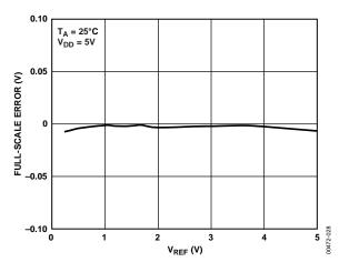
Figure 24. Full-Scale Error vs. V<sub>REF</sub> (Buffered)
