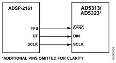
Figure 30. AD5313/AD5323 to ADSP-2161 Interface
