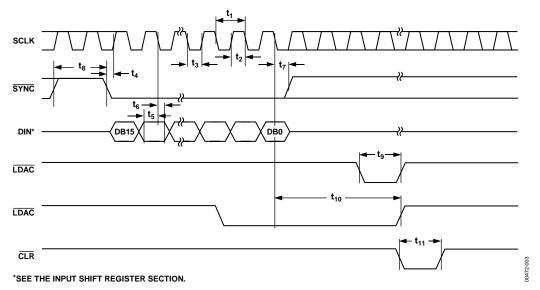
Figure 5. Serial Interface Timing Diagram
