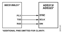
Figure 32. AD5313/AD5323 to 80C51/80L51 Interface
