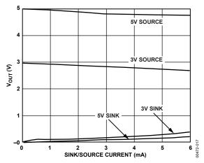
Figure 13. Source and Sink Current Capability
