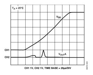
Figure 19. Power-On Reset to 0 V
