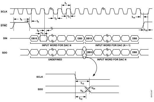
Figure 42. Daisy-Chaining Timing Diagram
