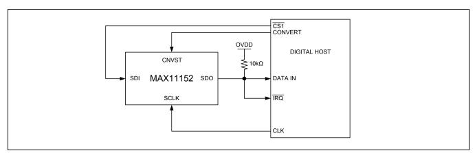
Figure 11. CS Mode 4-Wire with Busy Indicator Connection Diagram
