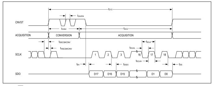
Figure 6. CS Mode 3-Wire, No-Busy Indicator Serial Interface Timing (SDI High)
