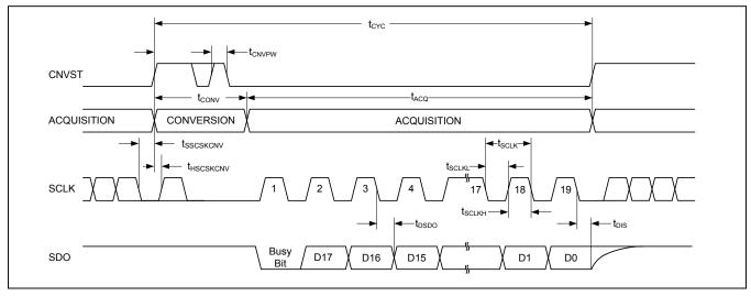
Figure 8. CS Mode 3-Wire With Busy Indicator Serial Interface Timing (SDI High)
