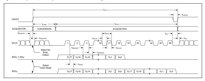
Figure 14. Daisy-Chain, No-Busy Indicator Mode Timing
