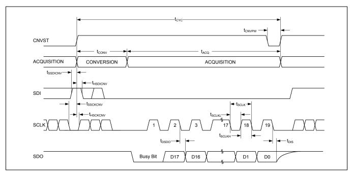
Figure 12. CS Mode 4-Wire with Busy Indicator Serial Interface Timing
