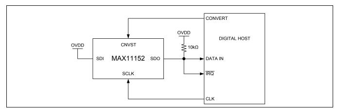
Figure 7. CS Mode 3-Wire With Busy Indicator Connection Diagram (SDI HIgh)
