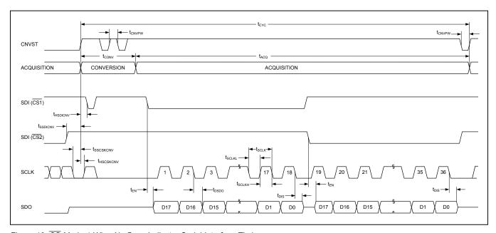
Figure 10. CS Mode 4-Wire, No-Busy Indicator Serial Interface Timing
