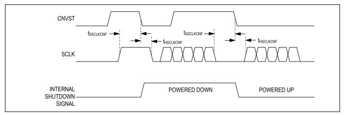
Figure 4. Entering and Exiting Shutdown Mode
