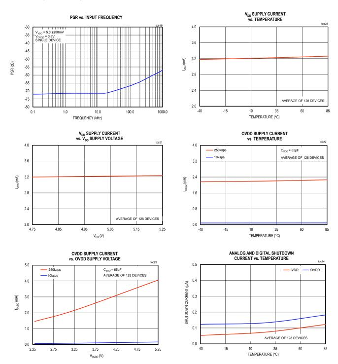
(V<sub>DD</sub> = 5.0V, V<sub>OVDD</sub> = 3.3V, f<sub>SAMPLE</sub> = 500kHz, V<sub>REF</sub> = 5V;  $T_A$  = +25°C, unless otherwise noted.)
