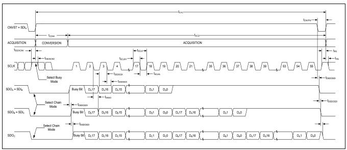
Figure 16. Daisy-Chain Mode with Busy Indicator Timing
