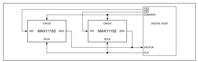
Figure 9. CS Mode 4-Wire, No-Busy Indicator Connection Diagram
