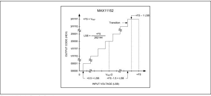
Figure 3. Unipolar Transfer Function
