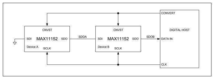
Figure 13. Daisy-Chain, No-Busy Indicator Mode Connection Diagram
