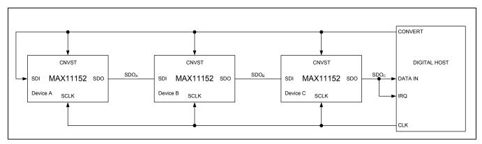
Figure 15. Daisy-Chain Mode with Busy Indicator Connection Diagram
