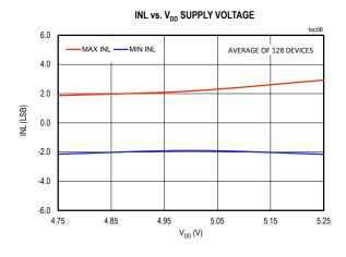
$(V_{DD}$  = 5.0V,  $V_{OVDD}$  = 3.3V,  $f_{SAMPLE}$  = 500kHz,  $V_{REF}$  = 5V;  $T_A$  = +25°C, unless otherwise noted.)
