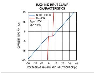
Figure 1. Input Clamp Characteristics
