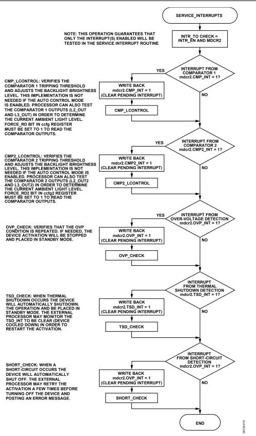
Figure 19. Service Interrupts Flowchart
