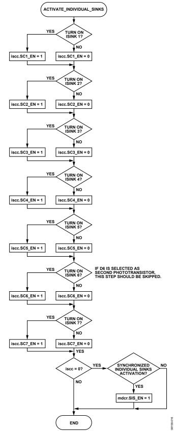
Figure 16. Activate Individual Sinks Flowchart
