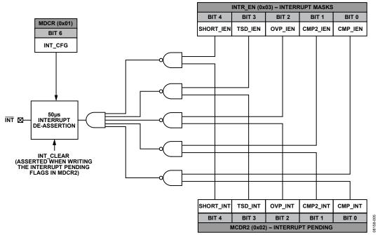
Figure 5. Interrupt Logic
