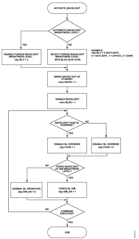
Figure 14. Activate Backlight Flowchart
