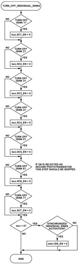
Figure 17. Turn Off Individual Sinks Flowchart
