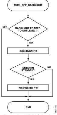
Figure 15. Turn Off Backlight Flowchart
