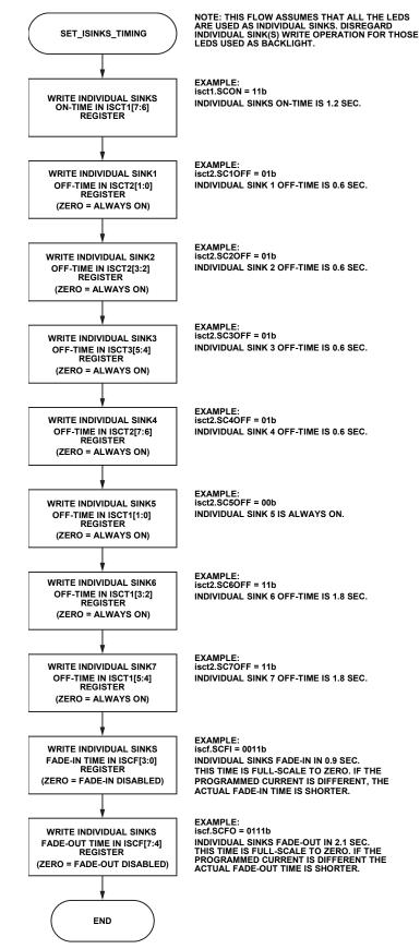
Figure 13. Set ISINKS Timing Flowchart
