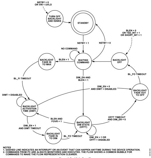
Figure 6. Backlight Data Flow
