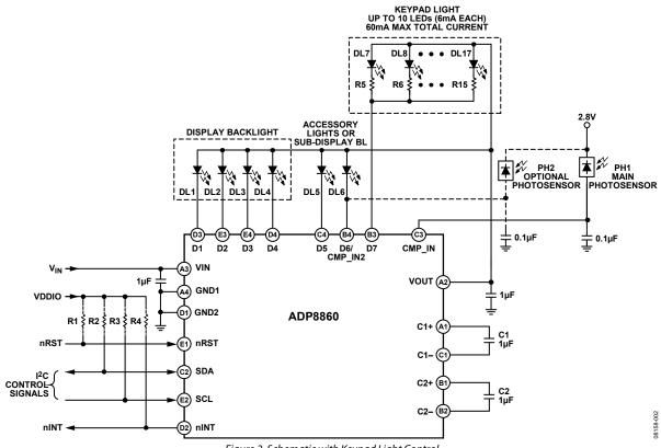
Figure 2. Schematic with Keypad Light Control
