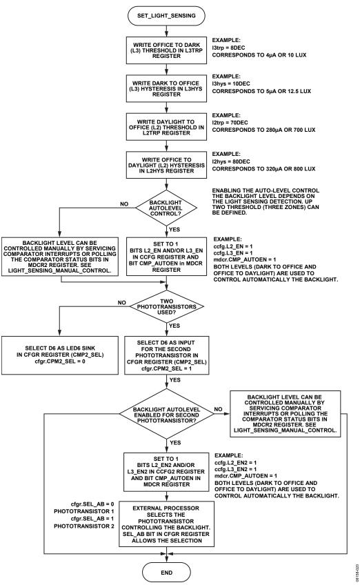
Figure 20. Set Light Sensing Flowchart
